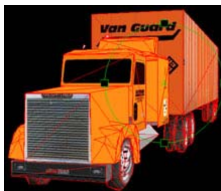
Optimized object faces removed up to 90 % 1834 faces 1140 points
